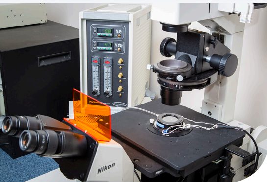
Works with 3rd party live cell microscopy stage chambers, such as the DH-35iL Culture Dish Incubator shown above.
