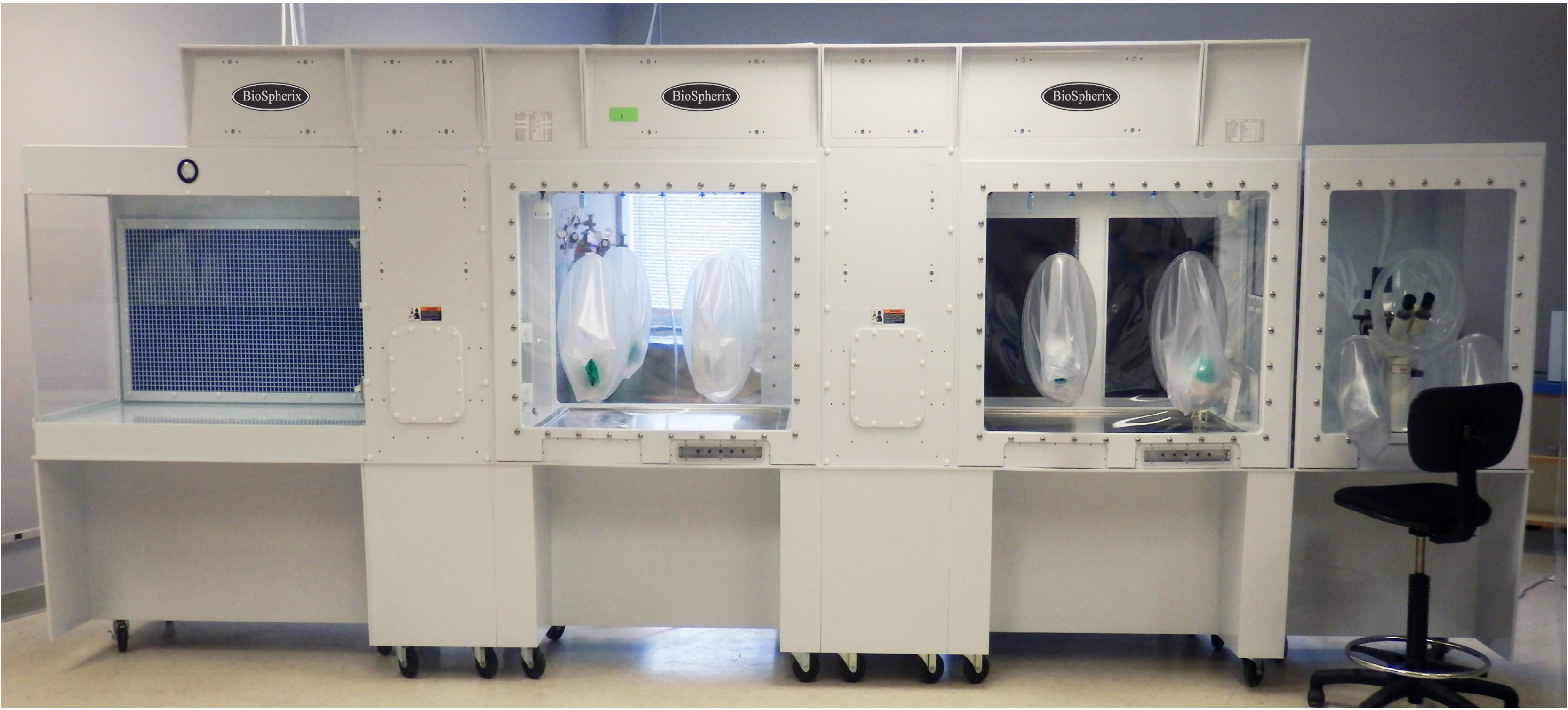
Figure 2. Experimental Design. All processes were performed in the Xvivo System. This system provides a completely controlled atmosphere from filtered, tanked gases. The atmosphere was continuously HEPA filtered and the temperature of the floor and air of each chamber can be controlled to constant 37°C. The black doors cover cell incubation chambers. Materials are disinfected in the laminar flow hood to the far left and brought into the system through buffer chamber air locks. Any entering room air was replaced with tanked gases before materials were imported. Probable risk surfaces inside the Xvivo and all imported materials were surface disinfected with SporKlenz RTU (Steris).
